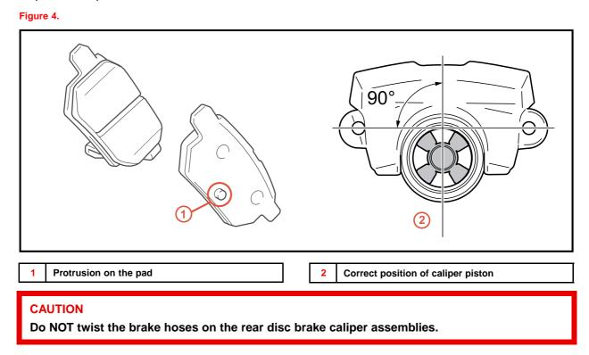
6. Install new rear brake anti-squeal shims with brake pads into the rear caliper assemblies brackets. Refer to (TIS), 2010 Prius Repair Manual:
