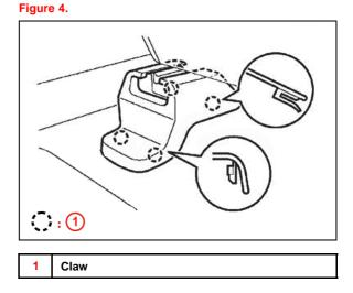
3. Remove the plastic rear seat track covers, use the Plastic Pry Tool to disengage the claws and carefully remove the plastic seat track covers.
