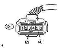
(a) Disconnect the throttle body assembly connector.
