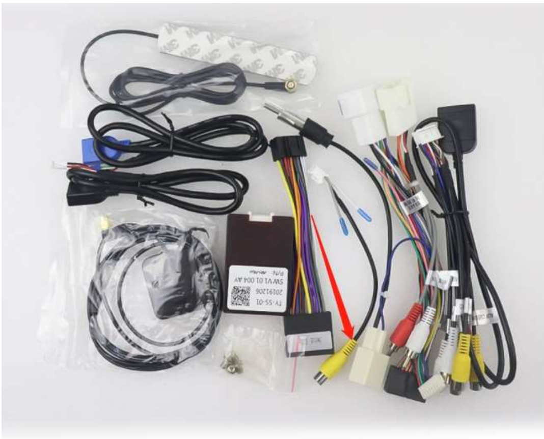
Figuur 7 Complete cable set with harness that supports a canbus.box
