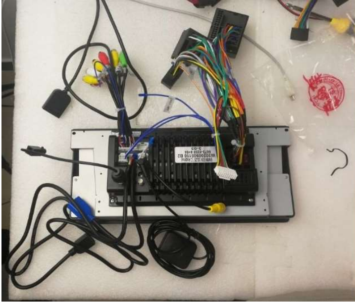
Figuur 22 All cables plugged in the new radio
