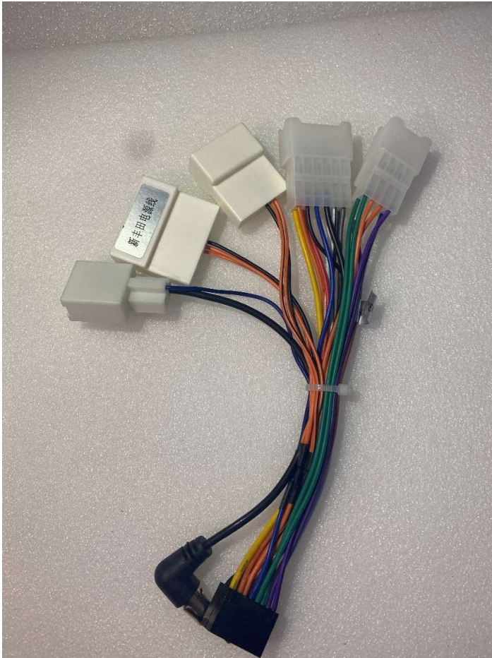
Figure 5 This harness connects the Toyota connectors to the android DIN connector.(Without canbus box support)
