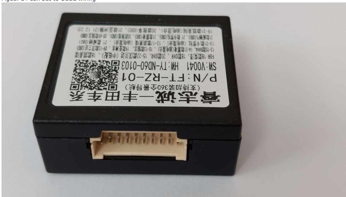
Figur 15 General Toyota Can Bus decoder
