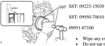
(b) Using SST and a hammer, tap in the oil seal until its surface is flush with the rear oil seal retainer edge.
