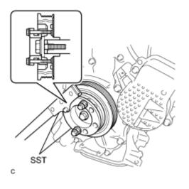
(b) Install the transmission input damper.
