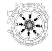
(c) Using several steps, uniformly install and tighten the 8 bolts in the sequence shown in the illustration.
