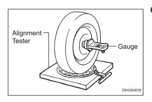
(e) Turn the right and left rack ends by an equal amount to adjust toe-in.
