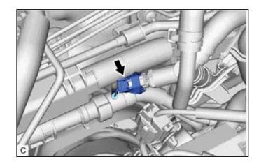
(b) Using a 19 mm union nut wrench, remove the engine coolant temperature sensor from the No. 2 water joint.
