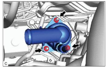
(2) Remove the gasket from the water inlet with thermostat sub-assembly.
