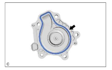
(c) Remove the gasket from the engine water pump assembly.
