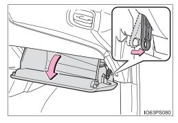
4 Push in each side of the glove box to disconnect the claws, and then slowly and fully open the glove box while supporting it.
