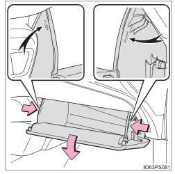
5 With the glove box fully open, slightly lift up the glove box and pull toward the seat to detach the bottom of the glove box.
