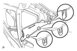
(a) Engage the 3 claws to install the front pillar garnish corner piece LH.
