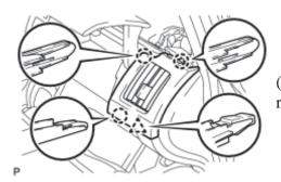
(a) Engage the 3 claws and clip to install the No. 2 instrument panel register.
