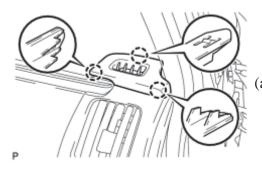
(a) Engage the 3 claws to install the No. 1 side defroster nozzle.
