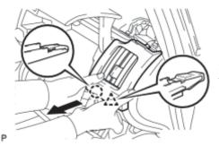
(a) Pull the No. 2 instrument panel register in the direction indicated by the arrow to disengage the claw and clip.
