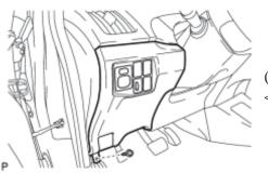
(e) Install the lower instrument panel finish panel assembly with the screw  $\langle C \rangle$ .
