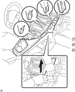
(b) Pull the lower center instrument cluster finish panel sub-assembly in the direction indicated by the arrow to disengage the 5 claws and remove the lower center instrument cluster finish panel sub-assembly.
