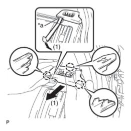
(b) Pull the No. 1 side defroster nozzle in the direction indicated by the arrow to disengage the 3 claws and remove the No. 1 side defroster nozzle.
