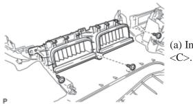
(a) Install the center instrument panel register assembly with the 3 screws
