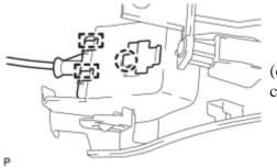
(c) Disengage the claw and 2 guides and disconnect the hood lock control cable.
