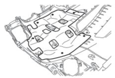
(a) Using hot-melt glue and install a new No. 2 instrument panel cushion as shown in the illustration.
