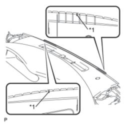
(a) Align the marking lines on the upper instrument panel with the ends of the No. 1 instrument panel cushion and install a new No. 1 instrument panel cushion as shown in the illustration.
