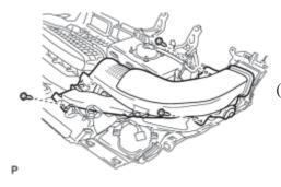
(a) Remove the 3 screws <C> and No. 2 heater to register duct.
