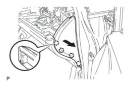
(a) Pull the instrument panel finish panel end RH in the direction indicated by the arrow to disengage the 4 claws.
