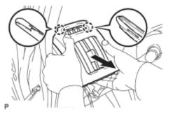
(b) Pull the No. 1 instrument panel register in the direction indicated by the arrow to disengage the 2 claws and remove the No. 1 instrument panel register.
