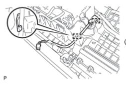
(a) Engage the 2 clamps to install the No. 5 instrument panel wire.
