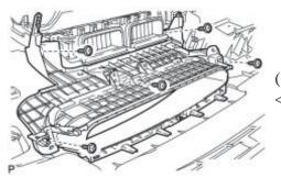
(a) Install the instrument cluster finish panel assembly with the 5 screws  $\langle C \rangle$ .
