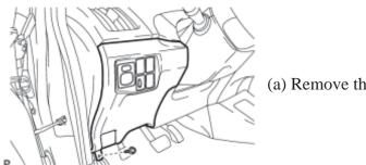
(a) Remove the screw  $\langle C \rangle$ .
