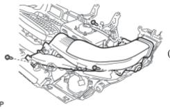
(a) Install the No. 2 heater to register duct with the 3 screws <C>.
