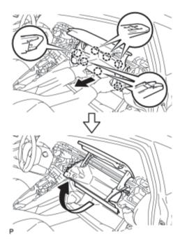
(c) Pull the glove compartment door in the direction indicated by the arrow to remove the glove compartment door.
