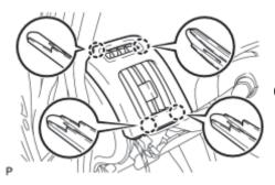
(a) Engage the 4 claws to install the No. 1 instrument panel register.
