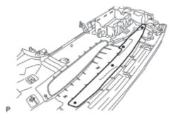
(a) Using hot-melt glue and install a new No. 4 instrument panel cushion as shown in the illustration.
