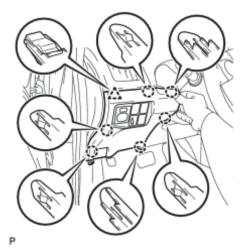
(b) Disengage the 6 claws and clip as shown in the illustration.
