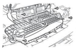
(a) Remove the 5 screws <C> and instrument cluster finish panel assembly.
