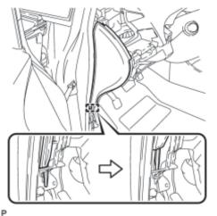
(c) Disengage the guide and remove the instrument panel finish panel end LH as shown in the illustration.
