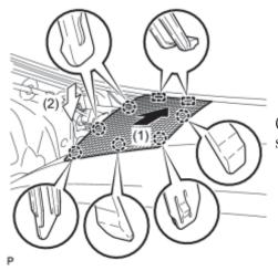
(a) Engage the 2 guides and 6 claws to install the No. 1 instrument panel speaker panel sub-assembly as shown in the illustration.
