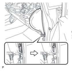
(c) Disengage the guide and remove the instrument panel finish panel end RH as shown in the illustration.
