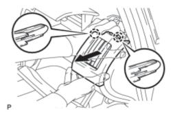
(b) Pull the No. 2 instrument panel register in the direction indicated by the arrow to disengage the 2 claws and remove the No. 2 instrument panel register.
