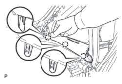
(a) Disengage the 3 claws and front pillar garnish corner piece RH as shown in the illustration.
