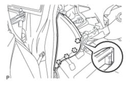
(c) Engage the 4 claws to install the instrument panel finish panel end LH.
