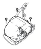
(a) Install the instrument panel cup holder with the 4 screws <C> to the lower center instrument cluster finish panel sub-assembly.
