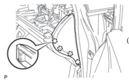
(c) Engage the 4 claws to install the instrument panel finish panel end RH.
