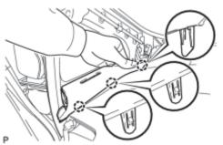
(a) Disengage the 3 claws and front pillar garnish corner piece LH as shown in the illustration.
