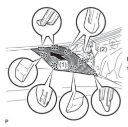
(a) Engage the 2 guides and 6 claws to install the No. 2 instrument panel speaker panel sub-assembly as shown in the illustration.
