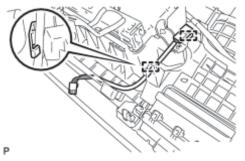
(a) Disengage the 2 clamps and remove the No. 5 instrument panel wire.
