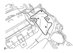
(a) Using hot-melt glue and install a new No. 5 instrument panel cushion as shown in the illustration.
