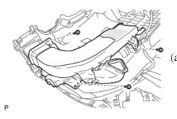
(a) Remove the 3 screws <C> and No. 3 heater to register duct.
