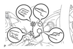
(a) Disengage the 4 claws to remove the No. 1 center instrument cluster finish panel.
