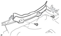
(a) Install the meter hood spacer with the 2 screws <C>.
