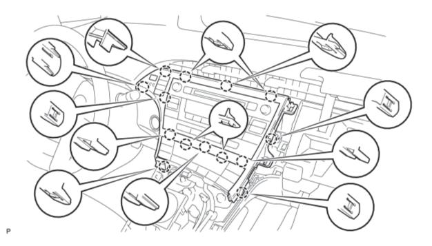
10. REMOVE UPPER INSTRUMENT PANEL FINISH PANEL SUB-ASSEMBLY
