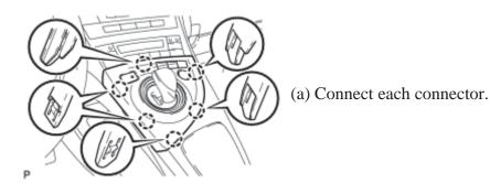
(b) Engage the 6 claws to install the integration control and panel assembly.
