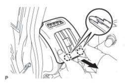
(a) Pull the No. 1 instrument panel register in the direction indicated by the arrow to disengage the 2 claws.
