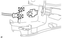
(c) Engage the 2 guides and claw to connect the hood lock control cable.
