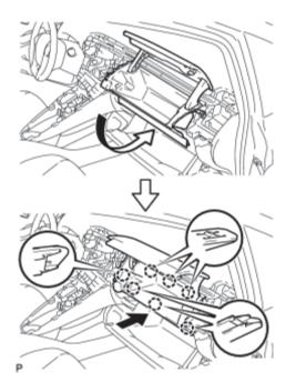
(c) Engage the 7 claws to install the glove compartment door.
