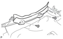
(a) Remove the 2 screws <C> and meter hood spacer.
