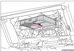
7 Remove the air conditioning filter from the filter case and replace it with a new one.
