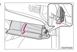
Push in each side of the glove box to disconnect the claws, and then slowly and fully open the glove box while supporting it.
