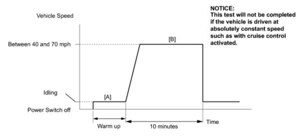
(Note: Even when vehicle stops during drive pattern, test can be resumed.)
