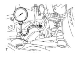
(b) Install the oil pressure gauge with the adapter.
