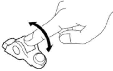
(a) Turn the roller by hand to check that it turns smoothly.
