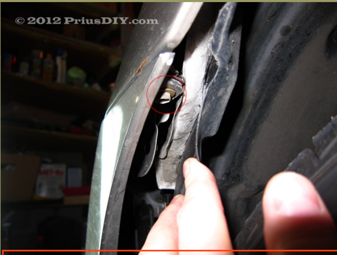
3) Pull back on the plastic fender and remove the 10mm bolt circled in red.
