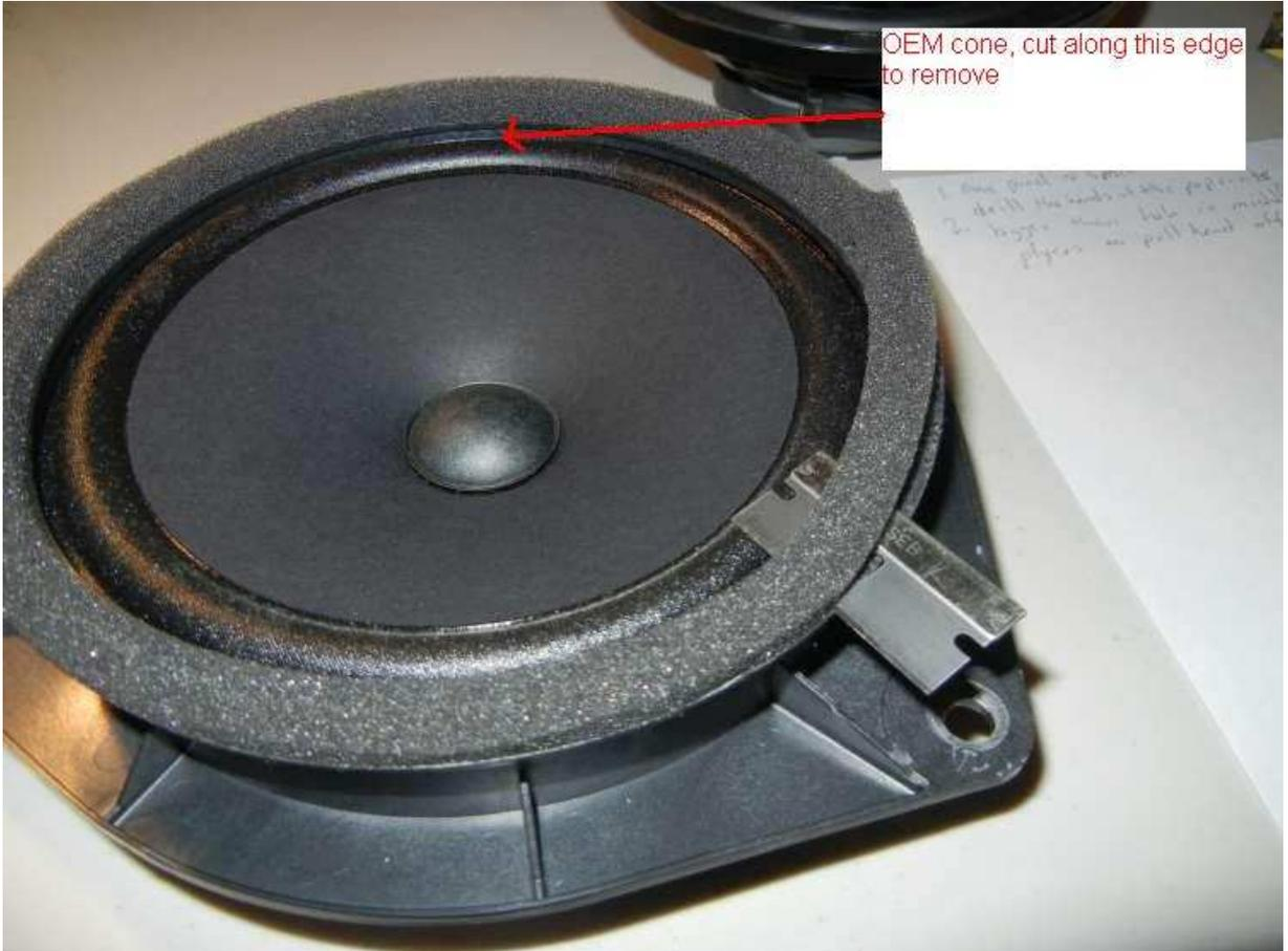
2. With the razor blade remove the paper cone of the speaker from the edges.
