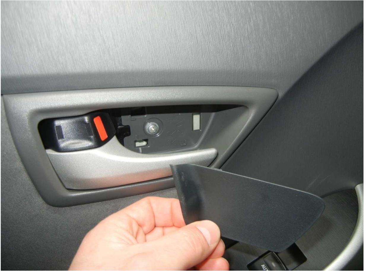
2. Grasp the panel at the opening at the bottom of the panel and yank firmly outward.
