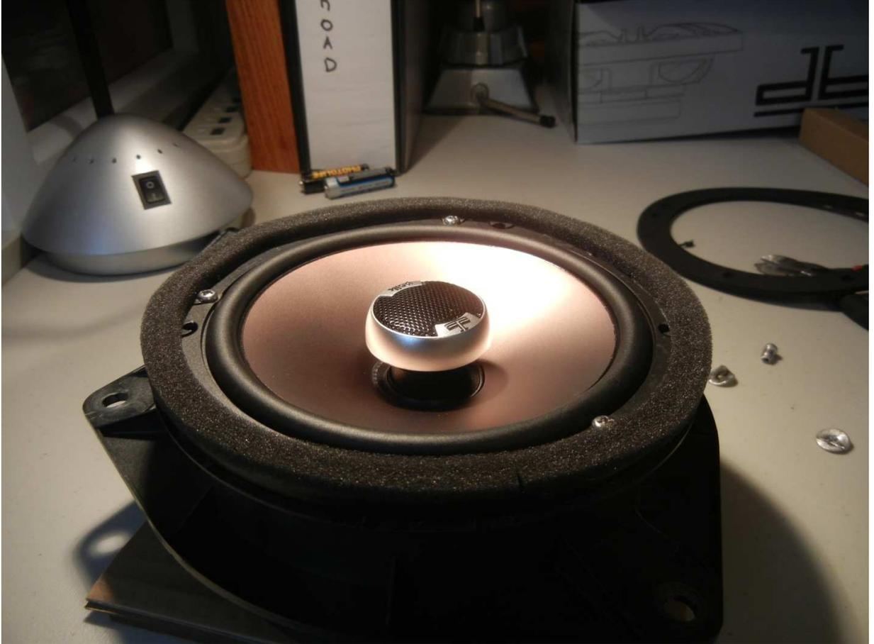
2. Place the speaker in the door hole. Make sure the speaker is centered by putting something to fill the three holes. I used the plastic inserts that came out when I removed the original rivets.
