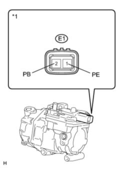
(i) Using a megohmmeter, measure the resistance according to the value(s) in the table below.
