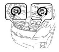
(1) Adjust the 2 cushion rubbers so that the heights of the hood and fender are aligned.
