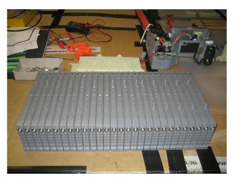
\* Assembling the pack in an up right position makes is much easier as the modules are packed closely to each other due to their own weight.
