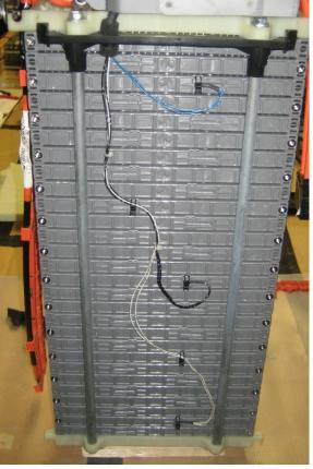
\* Don't forget the temperature sensors at the bottom
