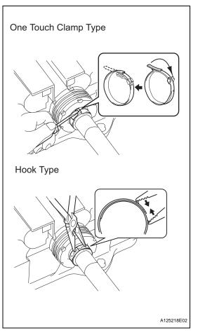
(a) Install the drive shaft damper to the outboard joint LH.
