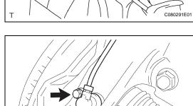
(b) Remove the bolt and front speed sensor from the steering knuckle.
