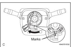
(b) Rotate the spiral cable clockwise approximately 2.5 turns to align the marks.
