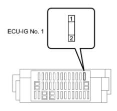
(a) Remove the ECU-IG No. 1 fuse from the instrument panel junction block.
