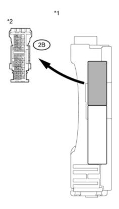
(a) Disconnect the driver side junction block assembly connector.
