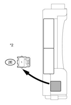
(a) Disconnect the driver side junction block assembly connector.
