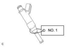
(c) For reinstallation, attach a tag or label to each injector shaft.
