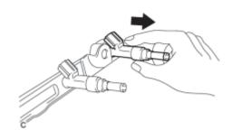
(a) Pull the 4 fuel injector assemblies out of the fuel delivery pipe sub-assembly.
