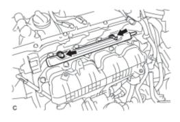
• Check that the fuel injector assemblies rotate smoothly after installing the fuel delivery pipe sub-assembly.
