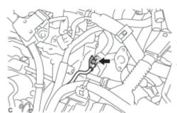
(b) Install the bolt to secure the fuel delivery pipe sub-assembly.
