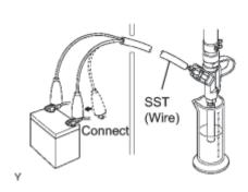
(6) Connect SST (wire) to the injector assembly and the battery for 15 seconds, and measure the injection volume with the graduated cylinder. Test each injector 2 or 3 times.
