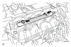
(b) Remove the 2 bolts and the fuel delivery pipe sub-assembly.
