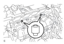
(a) Install the 2 No. 1 delivery pipe spacers onto the cylinder head.
