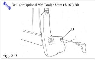
d) While holding inner mudguard tight to liner, drill 8mm (5/16") hole in liner at location D using part as a template (Fig. 2-3).
