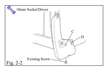
c) Reinstall existing screw in location C while holding part tight to panel and tighten (Fig. 2-2).
