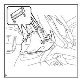
(c) Push the right and left sides of the lower steering column cover to disengage the 4 claws.
