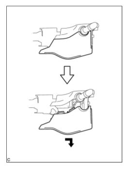
(i) Remove the lower steering column cover as shown in the illustration.
