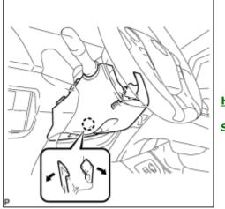
(d) Insert fingers into the opening of the tilt lever of the lower steering column cover to disengage the claw.
