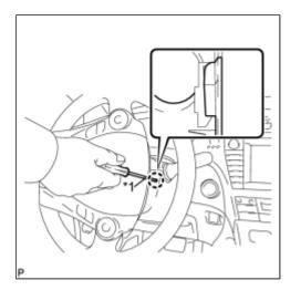
(e) Turn the steering wheel assembly to the right.
