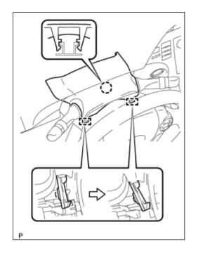
(a) Disengage the claw and 2 pins, and remove the upper steering column cover.
