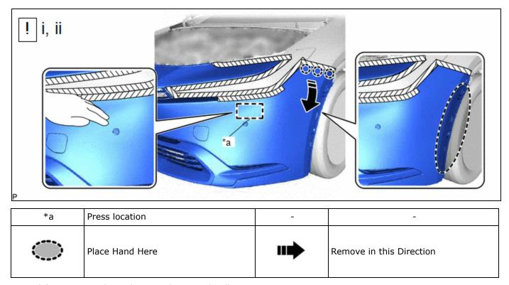
(1) Disengage the 3 claws as shown in the illustration.
