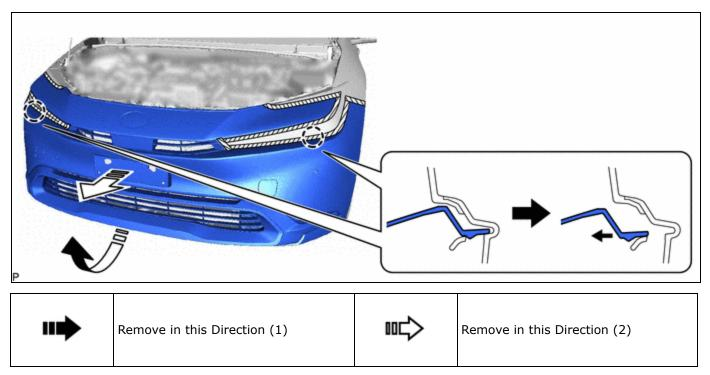
(1) Remove the 2 claws and remove the front bumper assembly as shown in the illustration.
