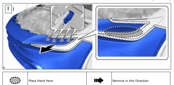
(1) Pull back the side of the front bumper assembly as shown in the illustration and disengage the 4 clips.
