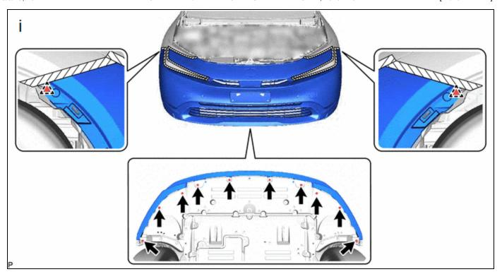
(1) Remove the 2 clips and 10 screws.
