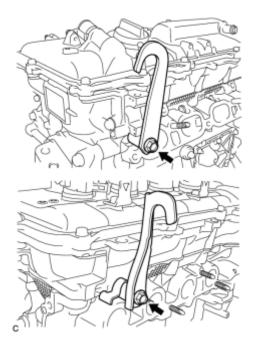
(g) Attach the sling device to the engine hangers and chain block.
