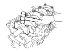
(h) Install the crankshaft bearing cap bolts.
