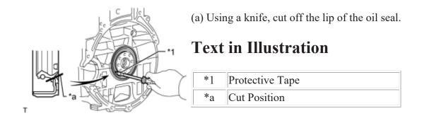
(b) Using a screwdriver with its tip wrapped with tape, pry out the oil seal.
