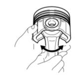
(e) Check the fitting condition between the piston and piston pin by trying to move the piston back and forth on the piston pin.
