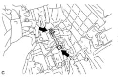
(d) Remove the bolt and nut, and separate the engine mounting insulator LH.
