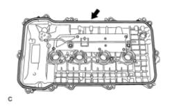
(a) Remove the cylinder head cover gasket.
