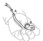
(c) Apply air into A. Check that air does not leak through B.
