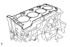
(a) Remove the cylinder head gasket.
