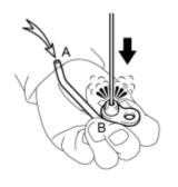
(d) Push the check valve while applying air into A. Check that air passes through B.
