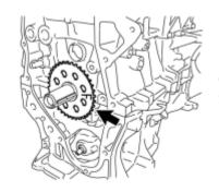
(a) Install the crankshaft position sensor plate with the "F" mark facing forward.
