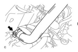
(a) Disconnect the outlet heater water hose.
