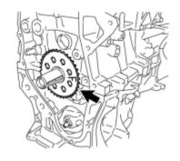
(a) Remove the crankshaft position sensor plate.
