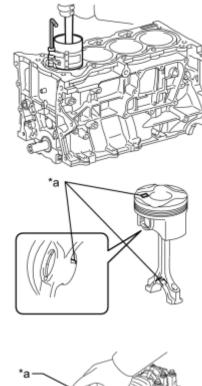
(c) Using a piston ring compressor, push the correctly numbered piston and connecting rod assembly into the cylinder with the front mark of the piston facing forward.
