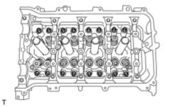
(a) Remove the 16 valve lash adjusters from the cylinder head.
