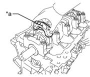
(d) Check that the front mark of the connecting rod cap is facing in the correct direction.
