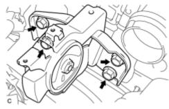
(a) Remove the 4 bolts and engine mounting insulator LH.
