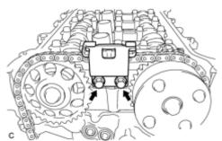
(a) Remove the 2 bolts and No. 2 chain vibration damper.
