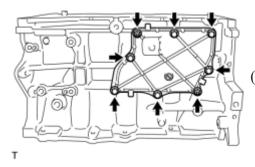
(a) Remove the 6 bolts and 2 nuts.
