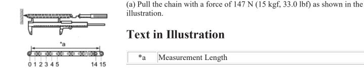
(b) Using a vernier caliper, measure the length of 15 links.
