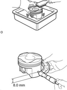
(c) Using a brush and solvent, thoroughly clean the piston.
