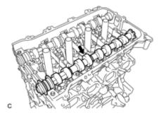
(a) Remove the camshaft.
