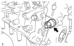
(b) Using a 24 mm deep socket wrench, install the engine oil pressure switch assembly.
