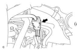
(a) Release the claw and remove the No. 1 fuel pipe clamp.
