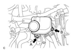
(a) Temporarily install bolt A to the inverter reserve tank assembly.
