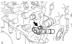
(b) Install the crankshaft position sensor with the bolt.
