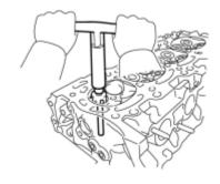
(a) Using a  $45^{\circ}$  cutter, resurface the valve seat so that the valve seat width is more than the specification.
