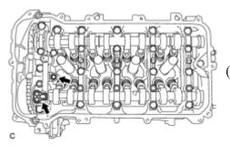
(b) Remove the 2 gaskets from the camshaft bearing cap.
