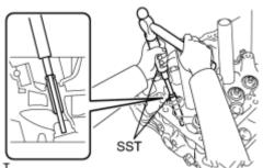
(c) Using SST and a hammer, tap out the guide bush.
