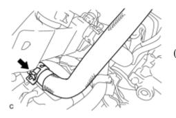
(a) Connect the outlet heater water hose with the clamp.
