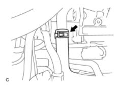
(a) Connect the No. 1 radiator hose with the clamp.
