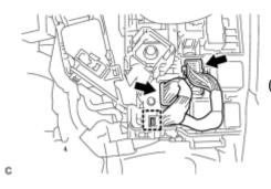
(d) Connect the wire harness to the engine room junction block.
