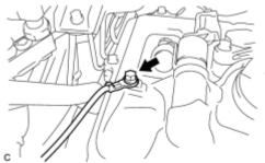
(e) Remove the bolt and disconnect the earth wire.
