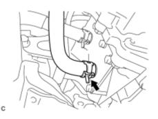
(a) Disconnect the No. 3 inverter cooling hose from the hybrid transaxle assembly.
