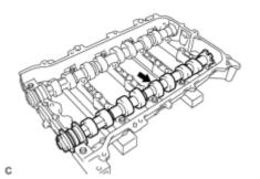
(c) Install the camshaft to the camshaft housing.
