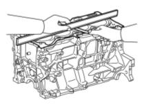
(a) Using a straightedge and feeler gauge, measure the warpage of the surface that contacts the cylinder head gasket.
