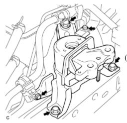
(a) Remove the 3 bolts and 2 cooler brackets.
