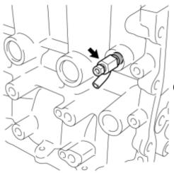
(a) Remove the drain cock plug from the drain cock.
