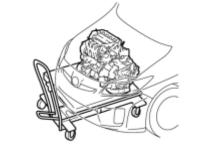
(c) Set the engine assembly with transaxle and front suspension crossmember on the engine lifter.
