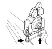
(a) Remove the 2 bolts and front engine mounting insulator.
