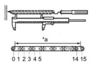
(a) Pull the chain with a force of 147 N (15 kgf, 33.0 lbf) as shown in the illustration.
