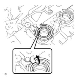
(b) Remove the 4 gaskets from the cylinder head cover.
