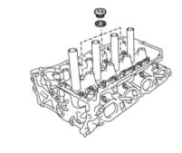
(a) Using a 10 mm straight hexagon wrench, remove the 3 screw plugs and 3 gaskets.
