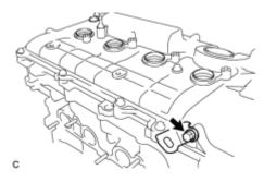
(a) Install the wiring harness clamp bracket with the bolt.
