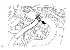
(a) Disconnect the No. 4 water by-pass hose from the radiator pipe assembly.
