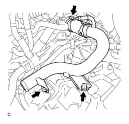
(b) Remove the 2 bolts and radiator pipe.
