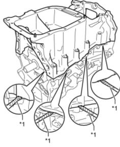
(b) Using a screwdriver, remove the stiffening crankcase by prying between the stiffening crankcase and cylinder block.
