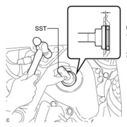
(b) Using SST and a hammer, tap in the oil seal until its surface is flush with the front oil seal retainer edge.
