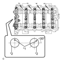
(b) Make sure of the marks and numbers on the camshaft bearing caps and place them in each proper position and direction.
