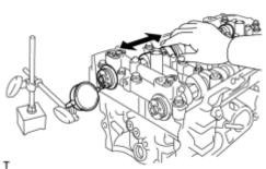
(b) Using a dial indicator, measure the thrust clearance while moving the camshaft back and forth.
