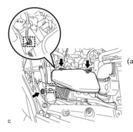
(a) Separate the water by-pass hose from the inlet air cleaner assembly.
