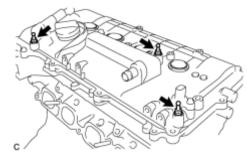
(a) Install the 3 engine cover joint bolts.
