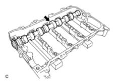
(c) Install the No. 2 camshaft to the camshaft housing.
