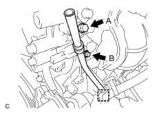
(c) Install the engine oil level dipstick guide with the 2 bolts.
