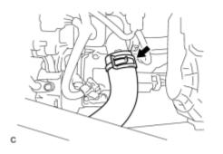
(a) Connect the No. 2 radiator hose with the clamp.
