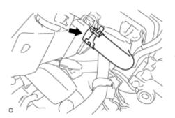
(a) Disconnect the inlet heater water hose.
