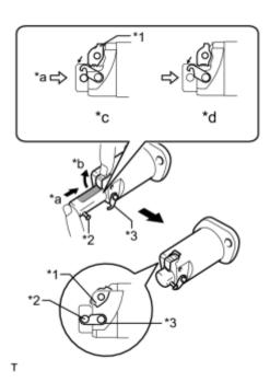
(a) Release the cam, and then fully push in the plunger and engage the hook to the pin so that the plunger is in the position shown in the illustration.
