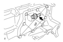
(a) Remove the ventilation valve sub-assembly.
