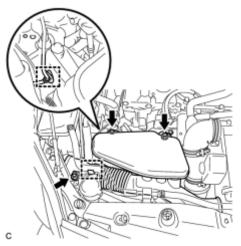
(a) Install the inlet air cleaner assembly with the 3 bolts.
