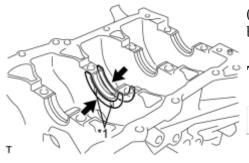
(a) Install the 2 thrust washers to the No. 3 journal position of the cylinder block with the oil grooves facing outward.
