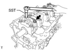
(1) Using SST, install and alternately tighten the bolts of the connecting rod cap in several steps.
