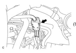
(b) Engage the claw and install the No. 1 fuel pipe clamp.
