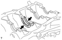
(a) Remove the 2 upper crankshaft thrust washers from the cylinder block.
