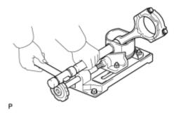
(c) Using a plastic-faced hammer and brass bar, lightly tap out the piston pin and remove the connecting rod.
