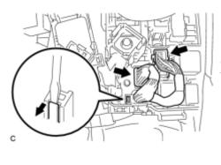
(c) Remove the 2 connectors and clamp from the engine room junction block and disconnect the wire harness.
