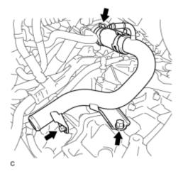
(b) Install the No. 3 radiator hose with the clamp.
