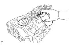
(a) Using a dye penetrant, check the intake ports, exhaust ports and cylinder surface for cracks.
