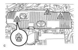
(a) Engage the 3 clips to install the cover.
