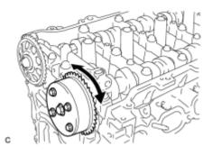
(f) Turn the camshaft timing gear within its movable range (26.5 to 28.5°) 2 or 3 times without turning it to the most retarded position. Make sure that the camshaft timing gear turns smoothly.
