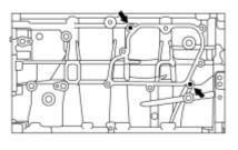
(a) Using an E6 "TORX" socket, install the stud bolts as shown in the illustration.
