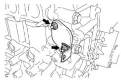
(a) Remove the 2 nuts, bracket, chain tensioner and gasket.
