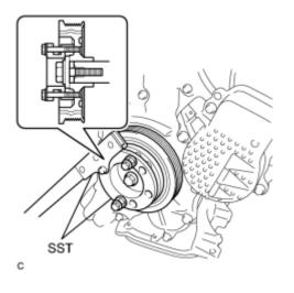
(b) Install the transmission input damper.
