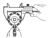
(a) Place the chain around the oil pump drive shaft gear.
