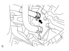
(a) Connect the No. 5 inverter cooling hose with the clamp.
