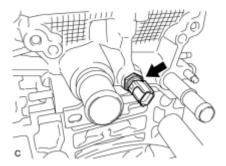
(a) Remove the engine coolant temperature sensor and gasket.
