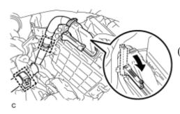
(f) Connect the connector to the ECM with the 2 clamps and lock lever.
