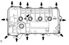
(a) Remove the 13 bolts, seal washer and cylinder head cover.
