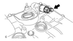
(a) Remove the bolt and camshaft timing oil control valve.
