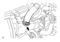
(a) Connect the heater hose with the clamp.
