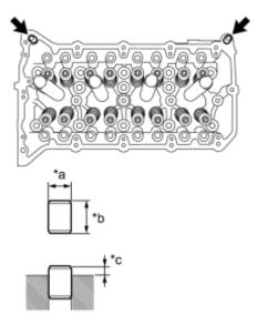
(b) Using a plastic-faced hammer, tap in a new ring pin to the specified protrusion height.
