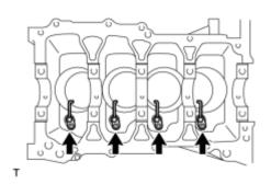
(a) Using a 5 mm socket hexagon wrench, remove the 4 bolts and 4 oil nozzles.
