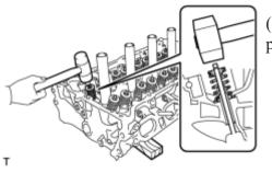
(e) Using a plastic-faced hammer, lightly tap the valve stem tip to ensure a proper fit.
