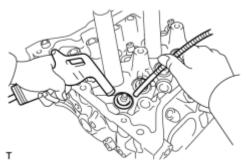
(a) Using compressed air and a Magnet Hand, remove the valve spring seats by blowing air onto them.
