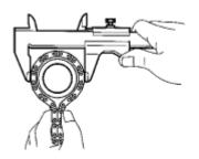
(b) Using a vernier caliper, measure the diameter of the crankshaft timing gear and chain.
