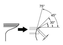
(b) Using  $30^{\circ}$  and  $75^{\circ}$  cutters, correct the valve seat so that the valve contacts the entire circumference of the seat. The contact should be in the center of the valve seat, and the valve seat width should be maintained within the specified range around the entire circumference of the seat.
