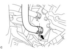
(a) Connect the No. 3 inverter cooling hose with the clamp.
