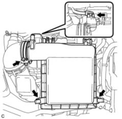
(a) Install the air cleaner cap sub-assembly with the 2 clamps and hose band.
