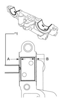
(c) Using a vernier caliper, measure the distance between the bearing cap edge and the camshaft bearing edge.
