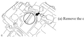
(a) Remove the oil filler cap.
