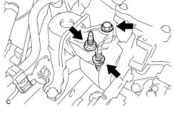
(c) Remove the bolt and 2 nuts, and separate the engine mounting insulator RH.
