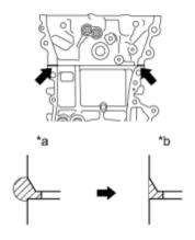
(d) After tightening the cylinder head bolts, wipe off the seal packing material seeped out from the contact surfaces between the cylinder head and cylinder block.
