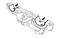
(a) Remove the 2 camshaft bearings
