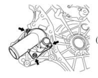
(a) Remove the bolt, 2 nuts, inlet water sub-assembly and gasket.
