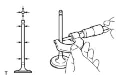
(b) Using a micrometer, measure the diameter of the valve stem.
