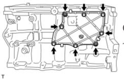
(b) Install the ventilation case with the 6 bolts and 2 nuts.
