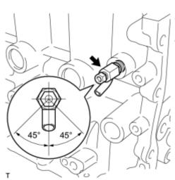
(b) Install the drain cock as shown in the illustration.
