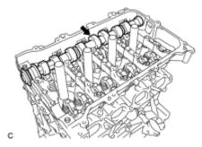
(a) Remove the No. 2 camshaft.
