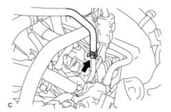
(a) Connect the No. 1 fuel vapor feed hose with the clamp.
