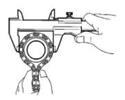
(b) Using a vernier caliper, measure the diameter of the oil pump drive gear and chain.Minimum gear diameter (with chain):
