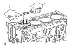
(a) Using a ridge reamer, remove all the carbon from the top of the cylinder.
