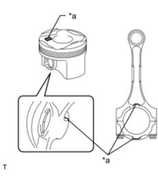
(c) Align the front marks of the piston and connecting rod, insert the connecting rod into the piston, and then push in the piston pin with your thumb until the pin comes into contact with the snap ring.
