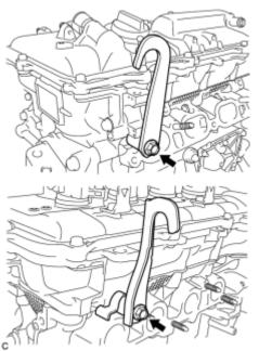
(b) Remove the 2 bolts and 2 engine hangers.
