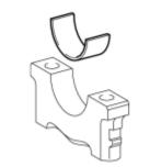
(b) Remove the 5 lower crankshaft bearings from the 5 crankshaft bearing caps.
