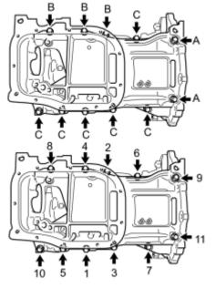
(b) Install the stiffening crankcase with the 11 bolts in the sequence shown in the illustration.
