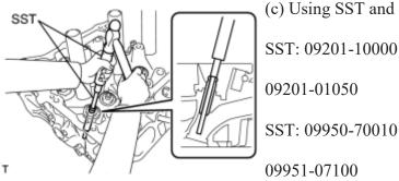
(c) Using SST and a hammer, tap out the guide bush.
