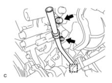
(a) Remove the engine oil level dipstick.
