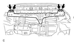
(b) Remove the 4 bolts and front crossmember sub-assembly.
