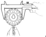
(a) Place the chain around the camshaft timing sprocket.
