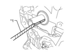
(a) Using a screwdriver, remove the 2 crankshaft timing gear keys.
