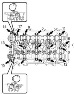
(c) Set the camshaft and No. 2 camshaft as shown in the illustration.
