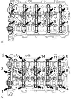
(a) Uniformly loosen and remove the 10 bearing cap bolts in the sequence shown in the illustration.
