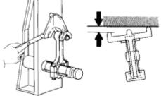
(2) Check for twist.Maximum twist:0.15 mm (0.00591 in.) per 100 mm (3.94 in.)
