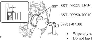
(b) Using SST and a hammer, tap in the oil seal until its surface is flush with the rear oil seal retainer edge.
