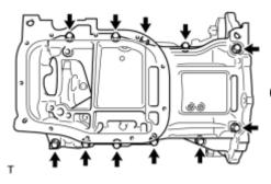
(a) Uniformly loosen and remove the 11 bolts.
