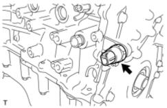
(a) Using a 24 mm deep socket wrench, remove the engine oil pressure switch assembly.
