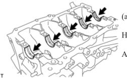
(a) Remove the 5 upper crankshaft bearings from the cylinder block.
