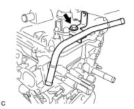
(a) Install the fuel vapor feed pipe with the bolt.
