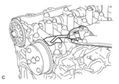
(d) Apply approximately 150 kPa (1.5 kgf/cm2, 22 psi) of air pressure to the hole pricked in procedure A to release the lock pin.
