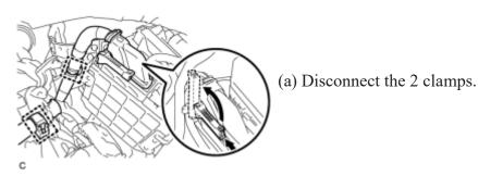
(b) Pull up the lever and disconnect the connector of the ECM.
