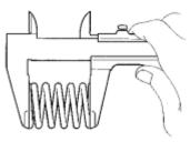
(a) Using a vernier caliper, measure the free length of the compression spring.
