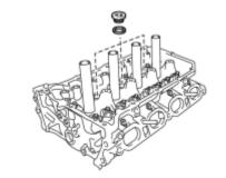
(a) Using a 10 mm straight hexagon wrench, install 3 new gaskets and the 3 straight screw plugs.
