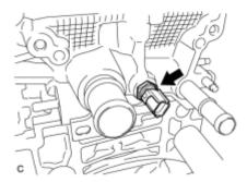
(a) Install a new gasket and the engine coolant temperature sensor.
