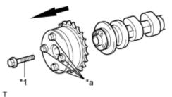
Keep the camshaft timing gear horizontal while removing it from the camshaft.
