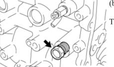
(b) Install the taper screw plug.
