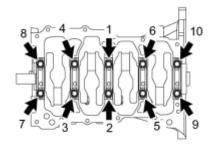
(1) Install and uniformly tighten the 10 crankshaft bearing cap bolts in the sequence shown in the illustration.
