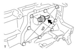
(b) Install the ventilation valve sub-assembly.
