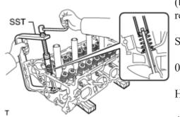
(b) Using SST and wooden blocks, compress and remove the valve retainer locks.
