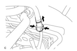
(b) Pinch the retainer as illustrated, then pull the fuel tube connector out of the pipe.
