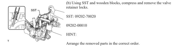
(c) Remove the retainer, valve spring and valve.
