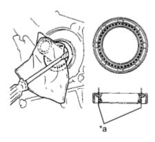
(b) Using a screwdriver with its tip wrapped with tape, pry out the oil seal.
