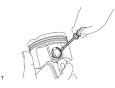
(a) Using a screwdriver, pry out the 2 snap rings.
