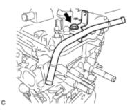
10. REMOVE FUEL DELIVERY PIPE SUB-ASSEMBLY\_
