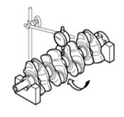
(1) Using a dial indicator and V-blocks, measure the circle runout as shown in the illustration.
