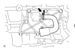
(a) Install the ventilation hose to the ventilation valve.
