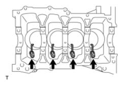
(a) Using a 5 mm socket hexagon wrench, install the 4 oil nozzles with the 4 bolts.
