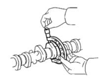
(1) Using a micrometer, measure the cam lobe height.
