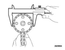
(b) Using a vernier caliper, measure the diameter of the camshaft timing gear assembly and chain.Minimum gear diameter (with chain):
