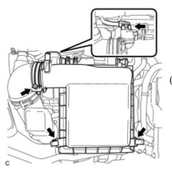
(a) Disconnect the air flow meter connector.
