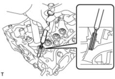
(h) Using a sharp 5.5 mm reamer, ream the guide bush to obtain the standard clearance between the guide bush and valve stem.
