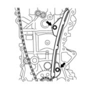
(a) Remove the 2 bolts and chain vibration damper.
