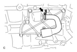
(a) Remove the ventilation hose from the ventilation valve.
