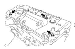
(a) Remove the 3 engine cover joint bolts.
