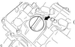
(a) Install the oil filler cap.
