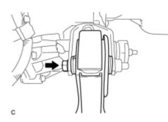
(a) Install the rear engine mounting insulator to the engine mounting bracket with the through bolt.
