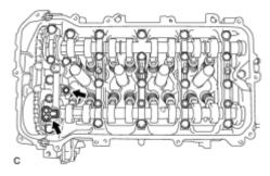
(a) Install 2 new gaskets to the camshaft bearing cap.
