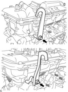
(a) Install the 2 engine hangers with the 2 bolts.
