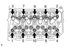
(a) Using a 10 mm bi-hexagon wrench, uniformly loosen and remove the 10 cylinder head bolts and 10 plate washers in several steps in the sequence shown in the illustration.
