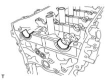
(a) Remove the 2 camshaft bearings.
