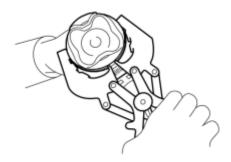
(b) Remove the oil ring and oil ring expander by hand.
