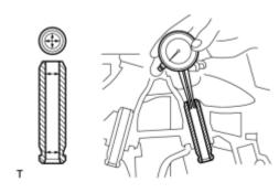
(a) Using a caliper gauge, measure the inside diameter of the guide bush.
