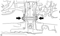
(i) Tighten the front engine mounting insulator with the bolt and nut.
