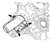
(a) Install a new gasket and the inlet water sub-assembly with the bolt and 2 nuts.
