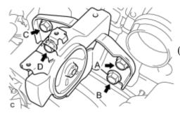
(a) Temporarily install bolt A to the engine mounting insulator LH.
