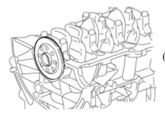
(a) Remove the engine rear oil seal from the cylinder block.
