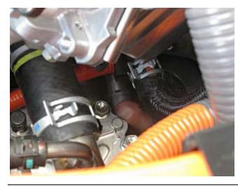
After a quick test-fit, the heater can be greased up with its included thermallyconductive goo, and inserted for real. There's Wayne's finger sliding 'er home.
