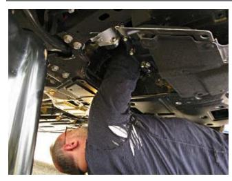
After removing the three fasteners from the access door in the underbelly panel and flipping it open, time to explore the rear corner of the engine block and determine how accessible the heater hole is. What's just out of the picture is my toe, holding the end of the door up because as it's just a flexible bit of plastic for the hinge, it really wants to flip back down and get in the way. A suitable clip or string to hold it fully open might be useful.
