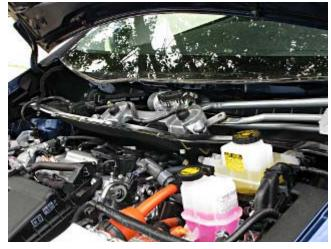
The wiper mechanism is a little different, but similarly bolted in with rubber spacers to give the whole assembly a little flex. The wire to the wiper motor goes up at the right side now.
