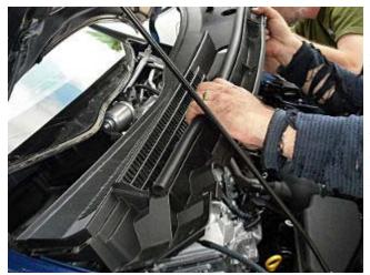
The long center plastic part is now one piece, avoiding the second-gen problem of having a seam in the middle that water could drip down through, missing the gutter piece and landing on the engine block below. The panel has claws that unclip from the gutter edge and the removal path unhooks downward and away from the windshield edge and then up, just like the second-gen version.
