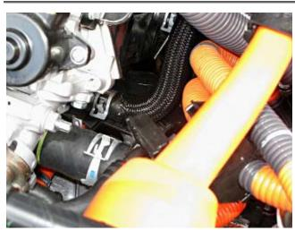
Both visual and physical access to the block-heater hole area, however, are somewhat flummoxed by a mess of cables in the way -- including the big scary orange ones for the battery and transaxle motors. Some of these need to be displaced a bit.
