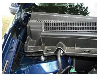
The new cowl cover is a little different. First, two little pieces at each side by the hood hinges need to be unclipped and removed -- uite easy. The wipers need to be unbolted and pulled off too, of course -- very similar to the second-gen.
