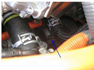
Note the orientation of the pins and flat side as it sits in place; flat side toward the front of the car. This is how it needs to sit to have the right-angle power wire fitting coming off toward the back of the car. The retainer clip on the heater also needs to be toward the back, which should be rotated around the right way before insertion.
