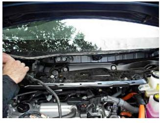
The 2010 gutter tray is much deeper front-to-back, and held in with several more bolts. There's also an extra bracket in the middle that helps hold up the wiper linkage, that needs to come out. After only 3000 miles there was already quite a bit of gunk in the tray, implying that routine removal of the cover and a bit of clean-out is a good idea especially if the car is parked under trees.
