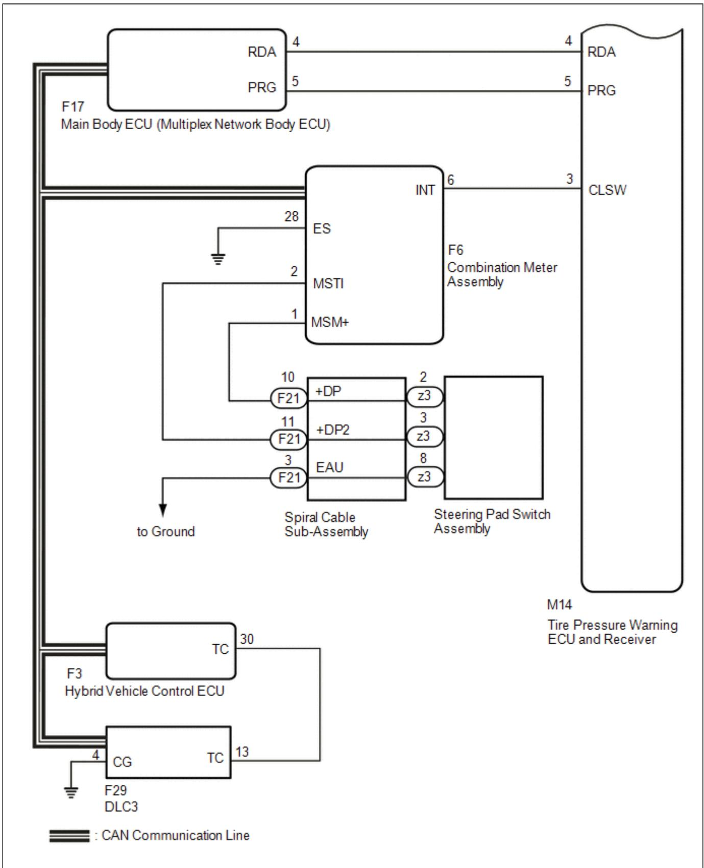
**HINT:** Each tire pressure warning valve and transmitter sends its transmitter ID, temperature and tire pressure information to the tire pressure warning ECU and receiver.
