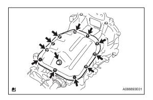
(d) Using several steps, install and uniformly tighten the 13 bolts in the sequence shown in the illustration.
