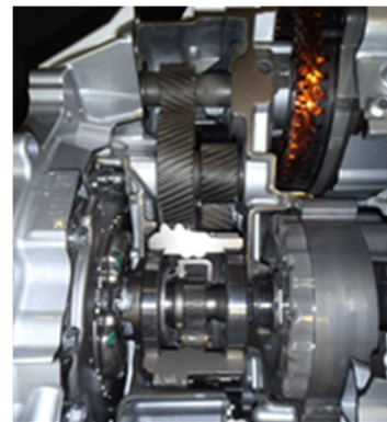
Figure 2: Cut Model of the Transaxle
