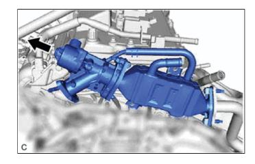
(f) Remove the EGR cooler gasket from the EGR pipe with cooler sub-assembly.
