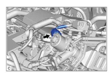
(b) Remove the 2 nuts and disconnect the EGR pipe with cooler sub-assembly from the exhaust manifold (TWC: Front Catalyst).
