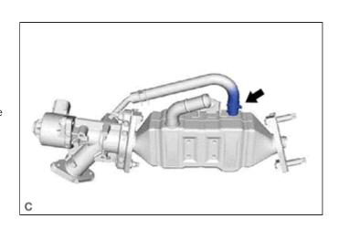
(h) Remove the 2 nuts and EGR pipe with cooler sub-assembly from the EGR valve assembly.
