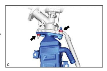
(i) Remove the EGR valve gasket from the EGR valve assembly.
