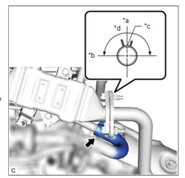
(a) Connect the No. 4 water by-pass hose to the EGR pipe with cooler sub-assembly and slide the clip to secure it.
