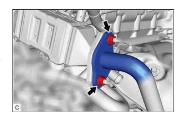
(j) Tighten the bolt and 2 nuts.
