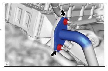
(c) Remove the bolt and 2 nuts and disconnect the EGR pipe with cooler sub-assembly with the EGR valve assembly from the cylinder head sub-assembly and camshaft housing sub-assembly.
