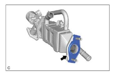
(g) Slide the clip and disconnect the No. 6 water by-pass hose from the EGR pipe with cooler sub-assembly.
