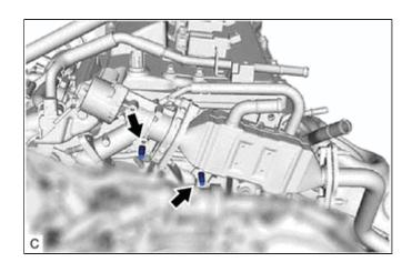
(e) Remove the EGR pipe with cooler sub-assembly with the EGR valve assembly.
