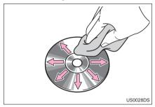
• To clean a disc: Wipe it with a soft, lintfree cloth that has been dampened with water. Wipe in a straight line from the centre to the edge of the disc (not in a circle). Do not use a conventional record cleaner or anti-static device.
