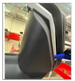
b. Remove the rear door rear bracket.
