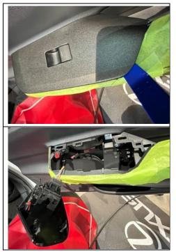
b. Remove the rear power window regulator switch assembly using a plastic trim tool.
