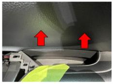
**10. INSTALL REAR DOOR TRIM BOARD SUB-ASSEMBLY** a. Slide the cover up until it snaps into place.
