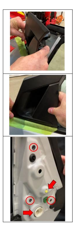
b. Install the <u>NEW</u> rear door outside handle assembly into the opening.
