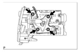
(a) Remove the 4 bolts and No. 1 radio bracket.
