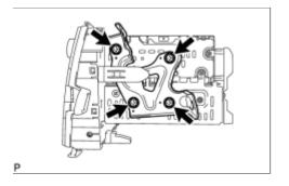
(a) Install the No. 1 radio bracket with the 4 bolts.
