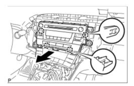
(b) Disengage the 4 claws as shown in the illustration.
