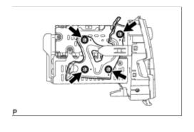
(a) Install the No. 2 radio bracket with the 4 bolts.
