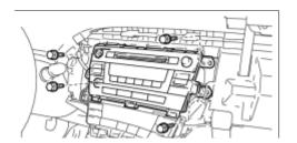
(c) Install the radio receiver with bracket with the 4 bolts.
