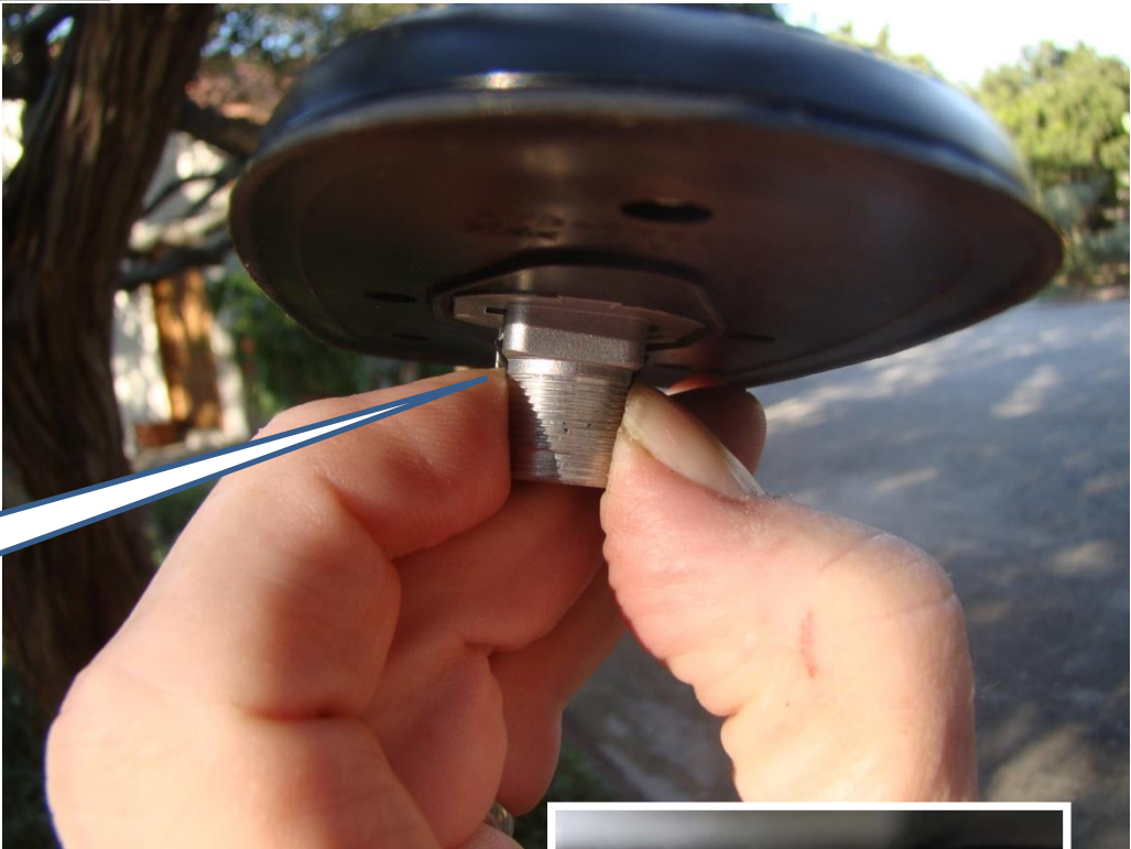
Press at Top of Threads after Nut Removed and Push Up Through Roof
