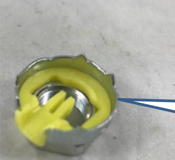
The Cable Exits through the Yellow Plastic Channel – Only the Nut Rotates
