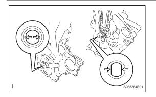
(c) Align the drive rotor spline of the oil pump with the rectangular portion of the crankshaft, then slide the oil pump into place.
