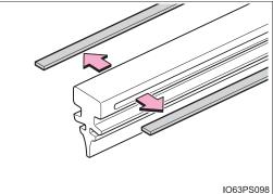
5 Insert the wiper rubber starting from the claw at the center of the wiper blade. Pass the wiper rubber through the 3 claws so that it sticks out from the stopper, and then pass the wiper rubber through the final remaining claw.
