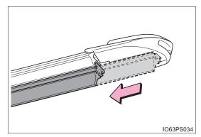
2 Pull out the end of the wiper rubber from the slit, and then pull out the rest of the wiper rubber.
