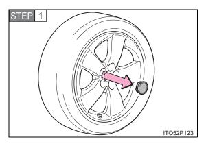
Vehicles with a 17 inch wheel: Before stowing the flat tire, remove the center wheel ornament by pushing from the reverse side.
