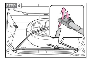
Pass the belt through the buckle and secure the tire firmly. Check that the belt is securely held by the buckle.
