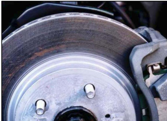
Figure 2. Slight Rust on Rotor (Easy to Remove by Braking)
