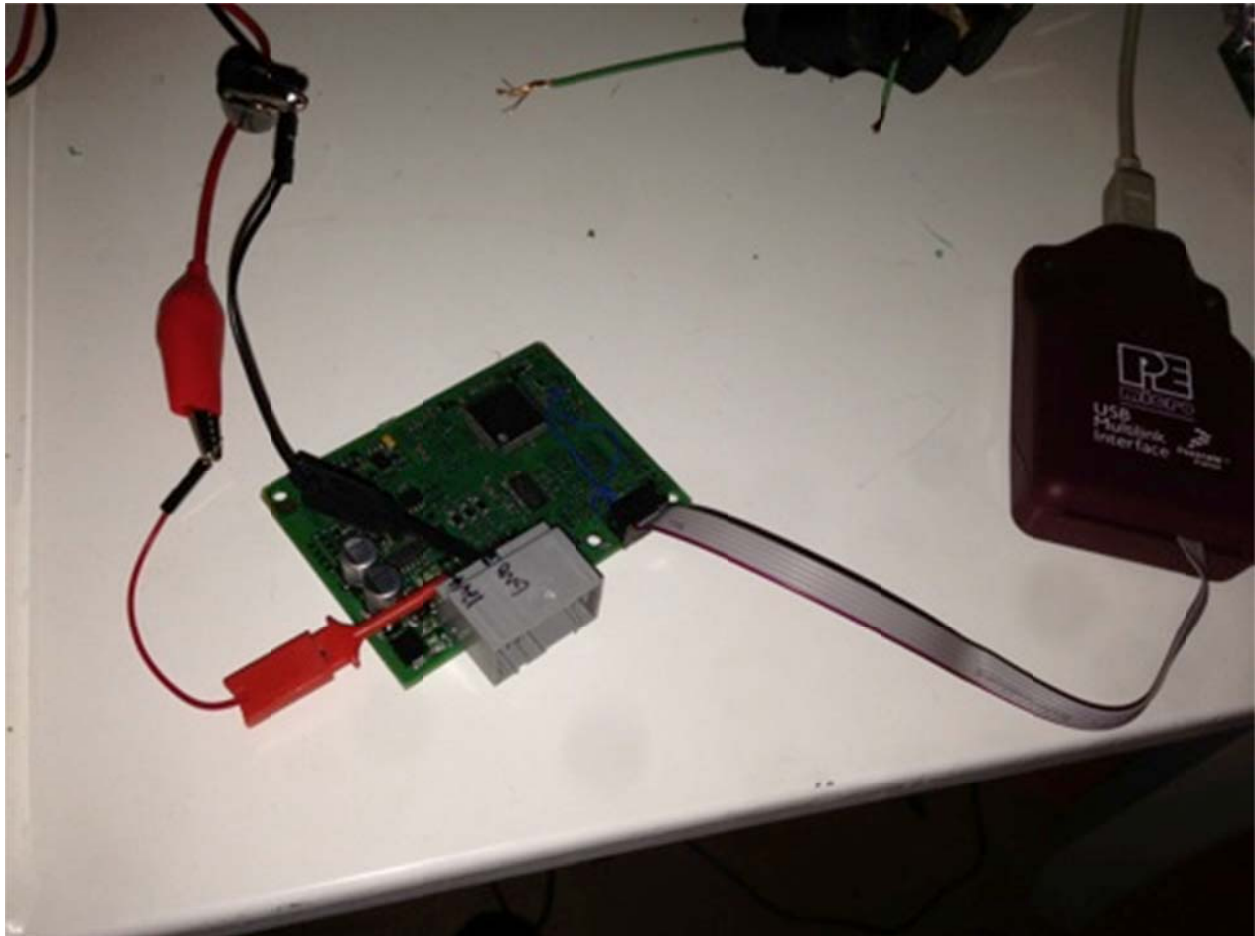
Figure 30: The PAM board connected to a BDM Multilink
