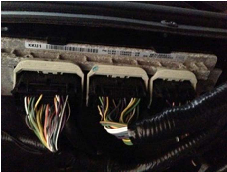
Figure 2: The Powertrain Control Module (PCM) from a 2010 Ford Escape.
