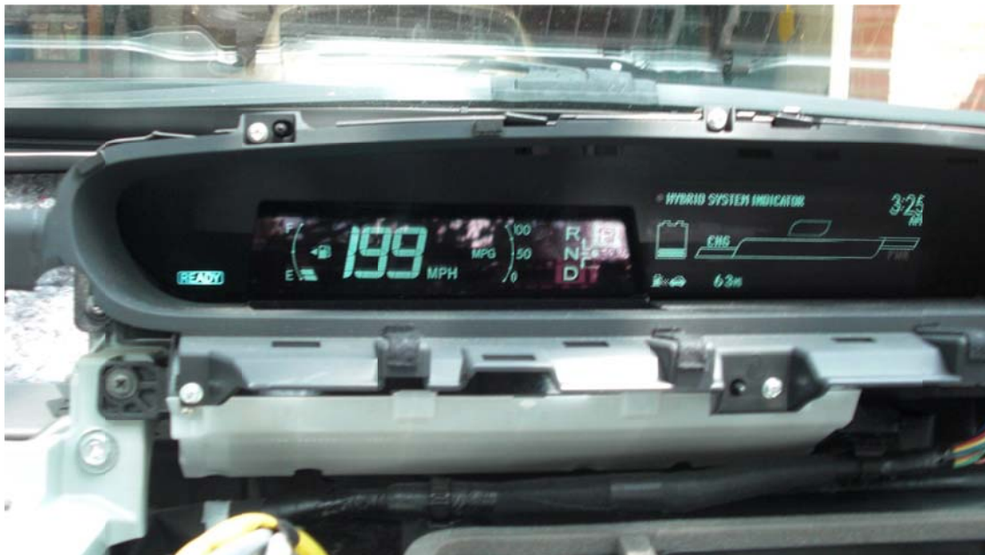
Figure 17: The speedometer can be altered to display any value.
