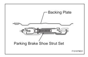
(c) Install the strut set as shown in the illustration.
