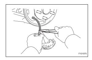
(c) Using needle-nose pliers, disconnect the parking brake cable, and remove the rear brake shoe.
