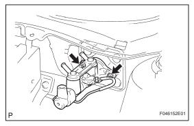
(g) Remove the 2 nuts, brake master cylinder gasket and brake master cylinder from the bracket.
