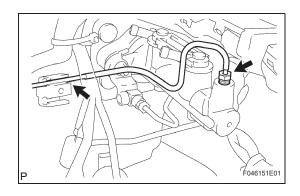
(f) Using SST, disconnect the No. 2 front brake tube from the clamp and brake master cylinder.SST 09023-00101
