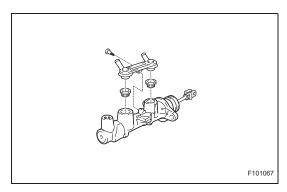
(i) Remove the screw, No. 1 brake master cylinder union and 2 grommets from the brake master cylinder.
