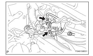
(c) Remove the 2 nuts, 2 bolts and brake stroke simulator cylinder with bracket.
