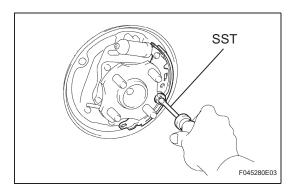
(b) Using SST, install the rear brake shoe, pin, shoe hold down spring and cup.
