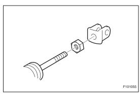
(j) Loosen the clevis lock nut and remove the brake master cylinder push rod clevis.
