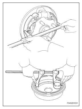
(b) Measure the brake drum inside diameter and the diameter of the brake shoes. Check that the difference between the diameter is the correct shoe clearance.
