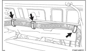
(b) Remove the 3 clamps from the outer front cowl top panel.
