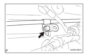
(c) Remove the clamp bolt from the No. 1 parking brake cable.
