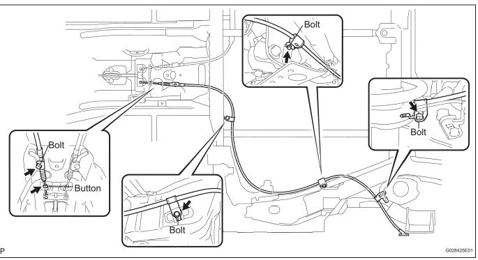
(c) Disconnect the No. 3 parking brake cable from the parking brake equalizer.
