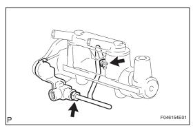
(h) Using SST, remove the brake tube and 2-way from the brake master cylinder.
