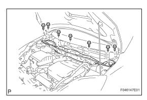
(c) Remove the 7 bolts and outer front cowl top panel.
