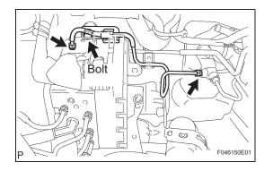
(g) Using SST, install the No. 1 front brake tube. SST 09023-00101
