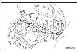
(b) Install the 3 clamps to the outer front cowl top panel.
