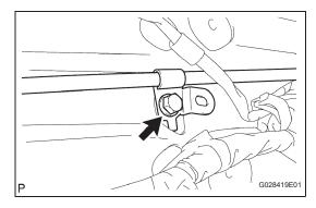
(e) Install the No. 1 parking brake cable to the floor with the clamp bolt.
