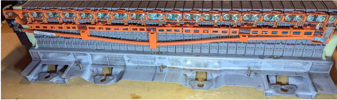
Figure 6 - HV battery front cell interface w. busbars
