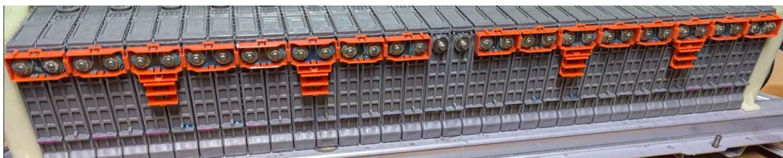
Figure 5 - HV battery rear cell interface w. busbars
