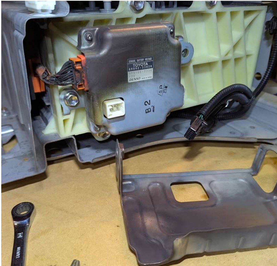
Figure 4 - Heat/carbon damage to module and cover plates
