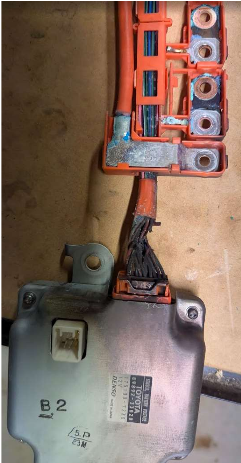
Figure 8 - 6 of 18 wires in sense harness have melted
