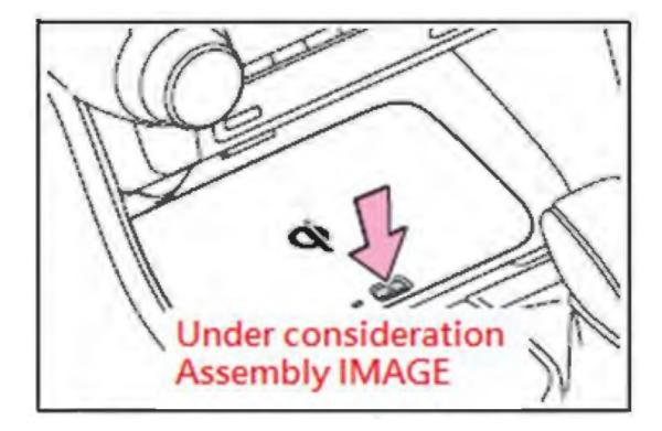
Place the charging side of the portable device down.
