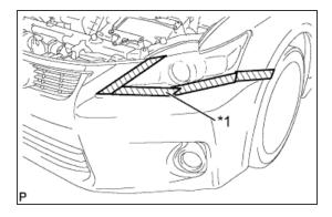
**b.** Using a screwdriver, turn the pins 90 degrees and remove the 2 pin hold clips.
