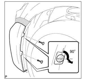
**c.** Remove the screw and front bumper seal bracket.
