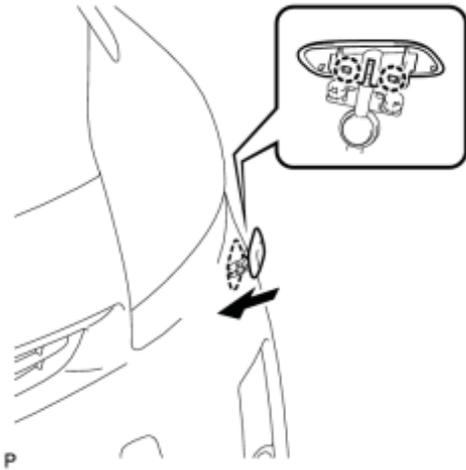
(a) Engage the 2 claws to install the headlight cleaner washer nozzle.
