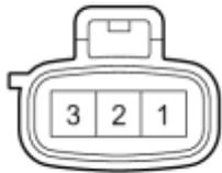
(b) Connect a battery positive (+) lead to terminal 2 of the headlight cleaner motor and pump, and a battery negative (-) lead to terminal 1.
