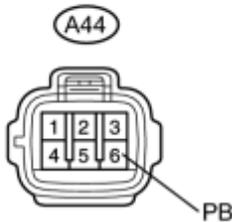
(b) Disconnect the A44 headlight cleaner control relay connector.
