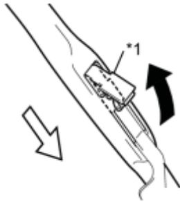
(a) Remove the holder of the front wiper blade as shown in the illustration.
