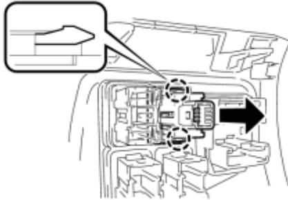
(a) Engage the 2 claws to install the headlight cleaner switch assembly as shown in the illustration.
