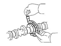
(1) Using a micrometer, measure the cam lobe height.
