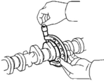
(1) Using a micrometer, measure the cam lobe height.
