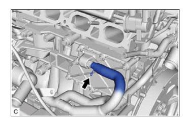
3. REMOVE PCV VALVE (VENTILATION VALVE SUB-ASSEMBLY)
