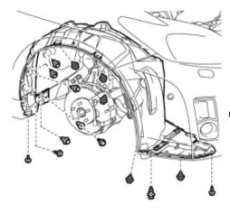
(b) Remove the 10 clips and 4 screws.
