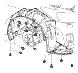
(a) Install a new grommet and the 4 screws.
