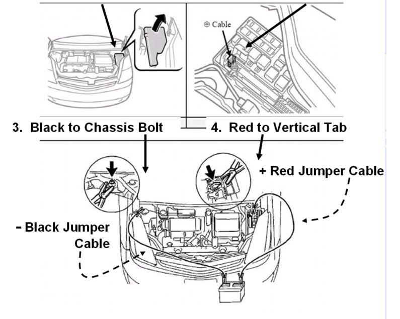
The 12V Auxiliary battery may be jump started if the vehicle does not start and the instrument cluster gauges are dim or off after depressing the brake pedal and pushing the power button.
